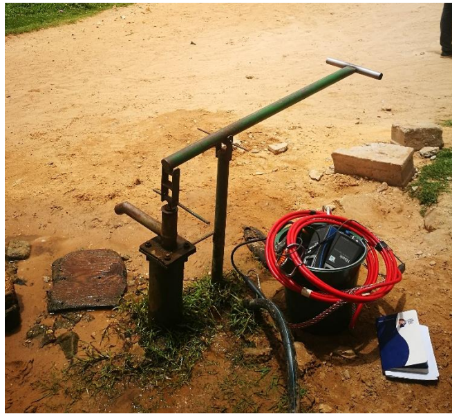
Figure 3: Fieldwork picture of TLF and CDOM sensors, which can be easily transported in a bucket
